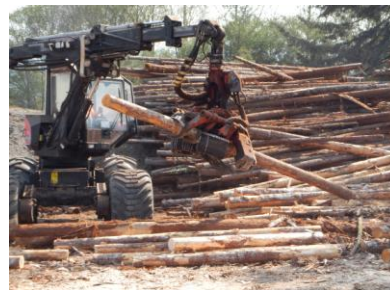
Processor sizing and sorting logs for the doweler
